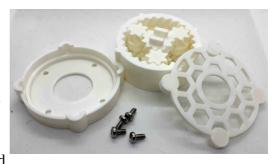
going through the rotary pump mechanism, it remains in the feed tube and is propelled along by bearings or more commonly rollers that push/pull small pulses of liquid along the tube. This means that nothing is in contact with the pump; everything stays in the tube. Makes for very easy cleaning and completely prevents cross contamination.
