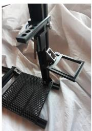
Above, funnel holder for filtering. On the left a view of the pump motor holder (square bit) and above it the bottle filling tube holder and fill switch.
