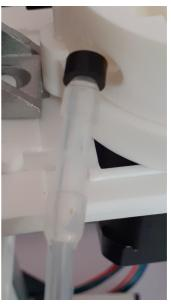
head and acts as a clamp for the tubing preventing it being taken through the pump. Its a nice little trick I learnt from a pump I had previously purchased, although in this case the collet I'm finding should be on the outgoing end which differs from the other pump which was on the supply side. Weird.
