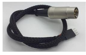
The 5 pin round DIN socket has four prongs at the other end to fit the pump or the stirrer motor as required.
